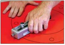
6. With slight downward pressure on cutter block and material, rotate cutter block clockwise to make cut. For thicker or hard to cut materials, make several passes to make cut. Or cut half way through material, turn over and complete cut.
