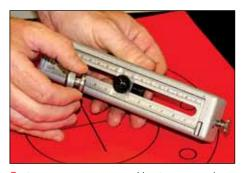
Remove pivot post assembly. Remove washer and install extension arm, thumb nut up.
