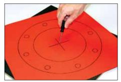
**2.** Create a pilot hole by piercing center of the gasket with piercing tool.
