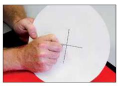
**2.** Push disc pin through center hole from bottom of template.
