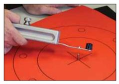
Place sleeved hole in extension bar over center pin in gasket material ensuring cutter block is lying flat on material.
