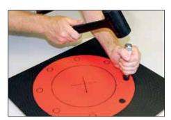
**7.** Reset cutter block for bolt holes and cut, or use hole punches to create bolt holes.
