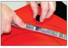
**4.** Use 0"-13" scale on cutter block. For example, to cut a 16" outside diameter gasket, add one Extension Bar. Match line through pivot post with the number "4" on scale. Secure with top nut.
