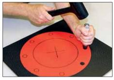
**8.** Reset cutter block for bolt holes and cut, or use hole punches to create bolt holes.
