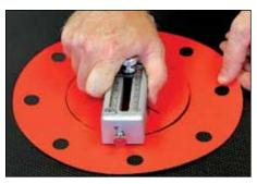
10. Make inside diameter cut for finished gasket.
