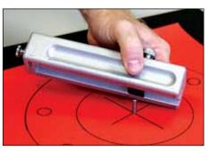
Position pivot post over center pin in gasket material ensuring cutter block is lying flat on gasket material.
