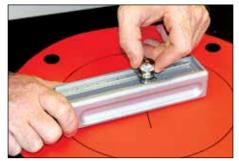
**8.** Reset cutter block for inside diameter dimension and cut.
