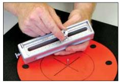
**9.** Reset cutter block for inside diameter dimension.
