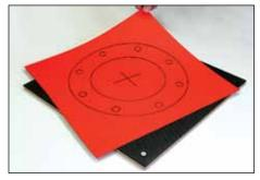
Lay out gasket outer diameter (OD), inner diameter (ID) and bolt holes on template or gasket material. (For information on drawing bolt holes visit WWW.ALLPAXCORP.COM)
