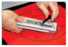
Reinstall pivot post assembly into cutter block. Place extension bar without stud in groove on bottom of cutter block with single, large hole in extension bar toward cutting blade.
