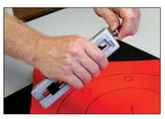
4. Loosen thumb screw of cutter block and position cutting blade so it protrudes slightly beyond thickness of gasket material. Tighten thumb screw.
