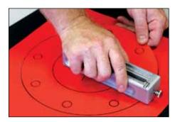
7. With slight downward pressure on cutting block and material, rotate cutter block clock wise to make cut. For thicker or hard to cut materials, make several passes to make cut. Or cut half way through material, turn over and complete cut. On difficult materials (hard, soft, etc.) consider using Easy Cutting Lubricant.
