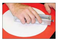
4. Use the disc pin as the pivot post to cut gasket material, as described above. Press down on the cardboard template to secure the gasket material.
