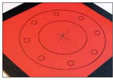
Place center pin into pilot hole in gasket material. Use appropriate length center pin for thickness of material being cut. Insert protruding center pin into recessed ferrule in middle of cutting board.
