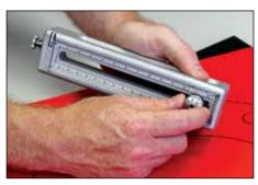
5. Loosen top nut and adjust pivot post to desired cutting diameter by matching pivot post indicator line with appropriate dimension of 0"- 13" scale. Secure with top nut.
