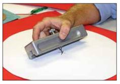
**3.** Place template on gasket material and push disc pin into gasket to make an indentation.
